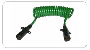
7P/12V coil - SAE J560 Primary, green cable, coil diameter: 100mm 1/8 + 2/10 + 4/12 ga.  $(1x 8.0mm^2 + 2x 5.0mm^2 + 4x 3.0mm^2)$
