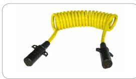
7P/12V coil - SAE J560 Auxiliary yellow cable, coil diameter: 100mm 1/8 + 2/10 + 4/12 ga.  $(1x 8.0mm^2 + 2x 5.0mm^2 + 4x 3.0mm^2)$
