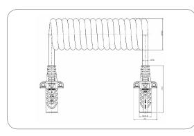
7P/12V Coiled Cable (Auxiliary, yellow) with molded plastic housing, molded anti kink protection Conductors: 1/8 + 2/10 + 4/12 ga. (1x 8.0mm<sup>2</sup> + 2x 5.0mm<sup>2</sup> + 4x 3.0mm<sup>2</sup>) Connectors: 2x7P/12V plugs, according to SAE J560-AUX (similar to ISO 3731)
