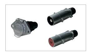
The 1-pin 24 V connector systems are mainly applied in supplement power supply for vehicle starting or attery charging in commercial vehicles and construction machines. The 1-pin 24 V connector systems are suitable for current intensity up to 300 A. They are used beside the known 15-and 7-pin 24 V connector systems. The system consists of two different 1-pin connectors (RED for supply and BLACK for common return).
