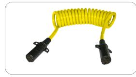
7P/12V coil - SAE J560 Auxiliary yellow cable, coil diameter: 100mm 1/8 + 2/10 + 4/12 ga. (1x 8.0mm² + 2x 5.0mm² + 4x 3.0mm²)
