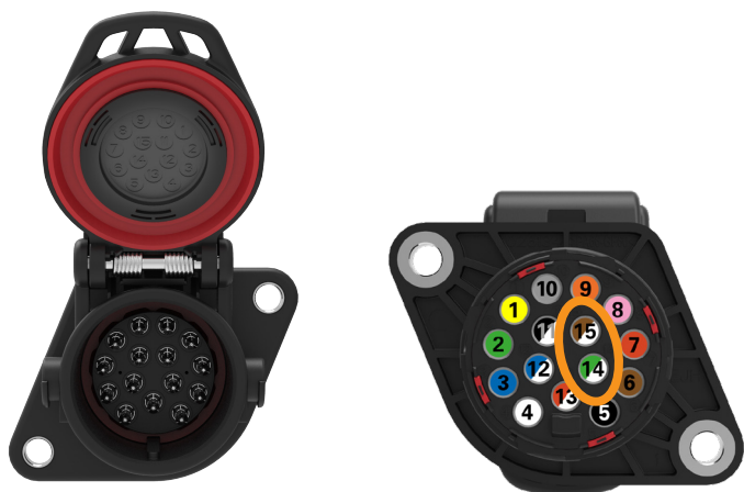
A trailer socket 15-pin 24V according to ISO 12098 with rear occupancy arrangement and CAN-BUS. The CAN-BUS data lines are located in chambers 14 and 15.
