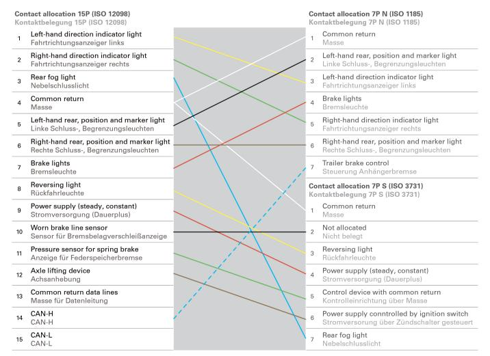
The cable between pole no. 14 of the 15P plug and pole no. 7 of the 7P pug is only allocated with the 15P plug and is placed insulated and back tied in 7P plug.
